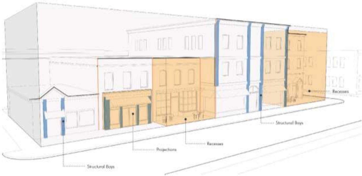
**Figure 20-E: Massing & Modulation – Vertical Components**
