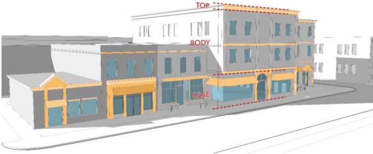
Figure 20-F: Massing & Modulation – Horizontal Components
