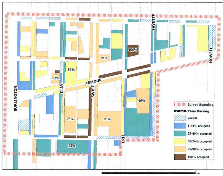
Parking Occupancy, 11am to 1pm
